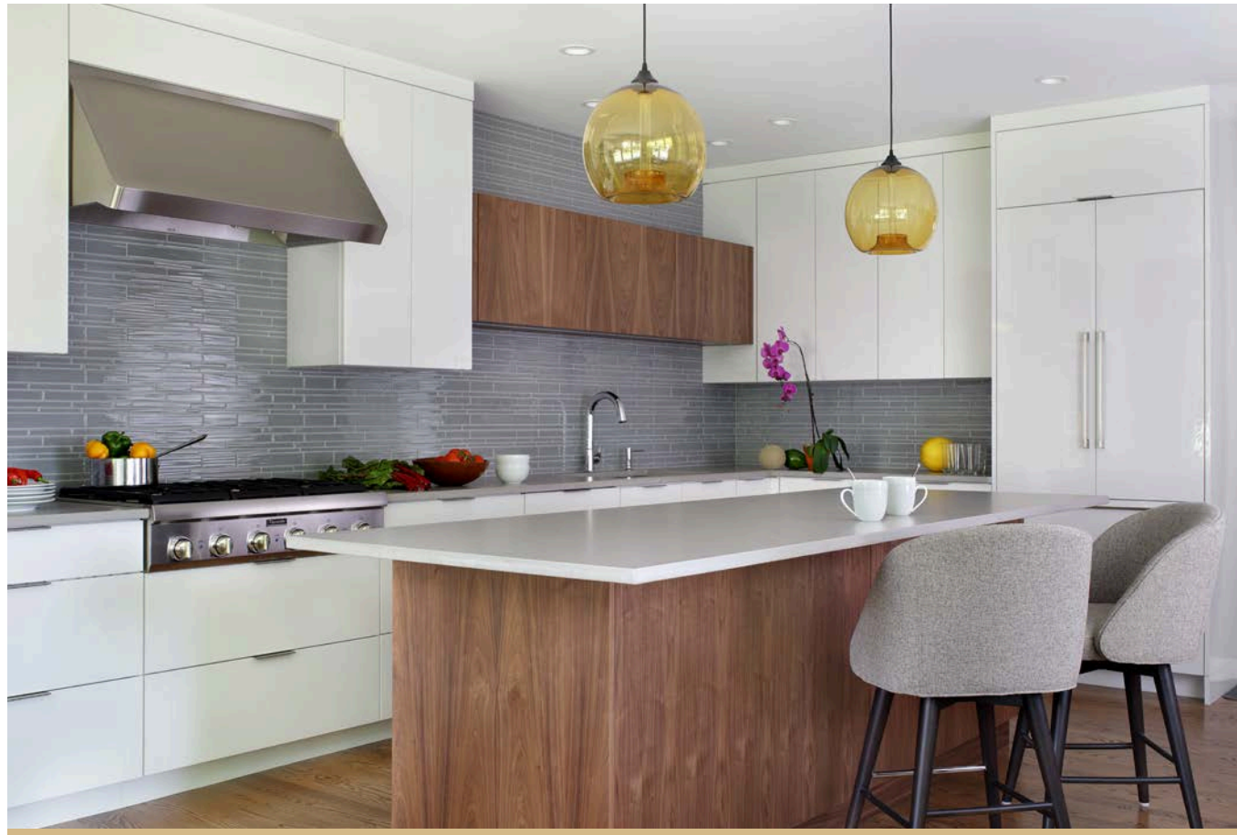
Base and Wall Cabinets » White Acrylic with Slab Doors in Full Overlay Island and Accent Wall Cabinet » Walnut with Natural Finish, Contempo Doors in Full Overlay
